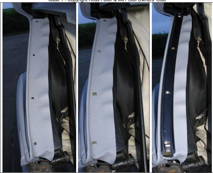
When gluing the rear side flaps, make sure the beaded edge of the hood is aligned nicely with the frame. I glued the rear side flaps on in two goes to get the alignment right (half of the flap with the roof closed, and half of it with it open). Open and close the hood as necessary to get the access required to screw in the screws of the seal brackets.
