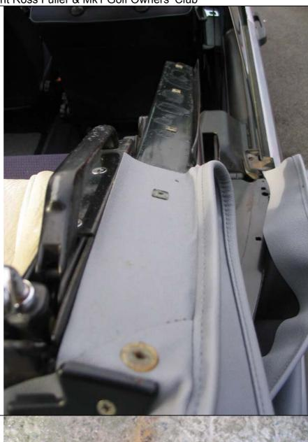
Then stick new gaskets to the side seal brackets and refit the brackets to the frame.
