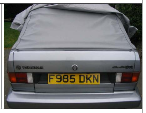
Also ensure the beading of the side flaps on the rear quarter of the hood just fit to the frame of the rear side window. It's a tricky process, and frustrating, but persevere and you'll get there...
