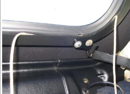
...while you from inside the car, pull the cord so that the lip of the seal gets pulled over the window frame. Go along the bottom of the window, up the sides, and finish at one of the top corners.
