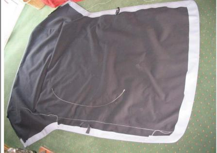
Some hoods (often mohair) come with excess material on the rear perimeter of the hood than needs trimming off along the line of the beading before fitting. I don't have any more detail on this.
