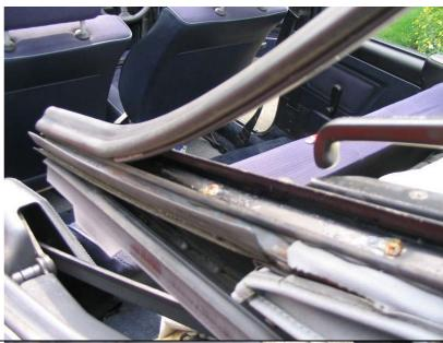
The front one has a screw to remove but after that's taken out the seals can just be pulled off. Do this carefully so the black plastic clips at the ends of the seal brackets don't snap.
