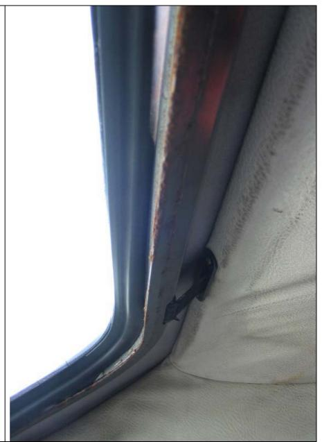
Use a screwdriver to lever out the staples that attach the hood to the window frame ...
