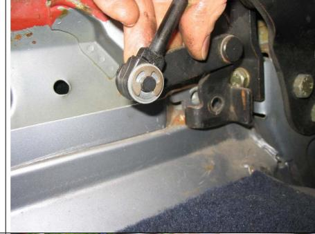
Position an open ended 5mm spanner on the rear cable itself to stop the cable twisting – allowing it to twist will snap the cable, keeping it intact will save a few quid. Its best to use a 10mm ratchet spanner to undo the nuts on the ends of the cable as access is tight.
