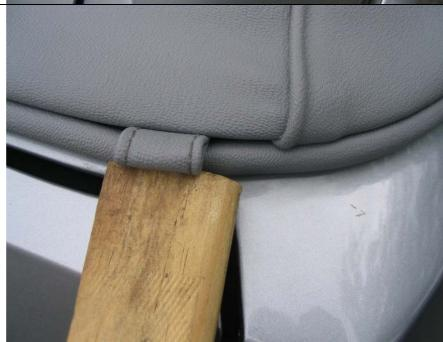
Finish off at the sides and poke the cable right up inside the lip.
