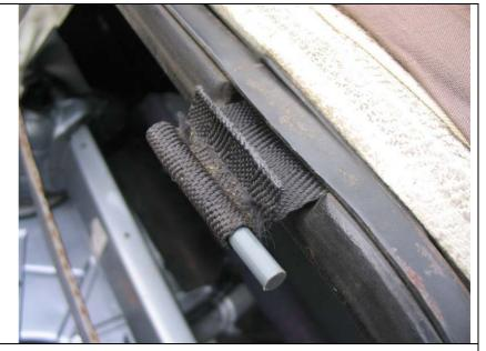
Close and latch the top. Make any repairs to the insulation layer that maybe needed. Now's the time to replace the layer and headliner if you need to (not covered here).
