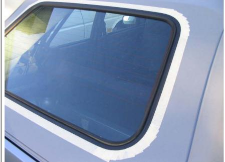
Then finally run a bead of silicone sealant between the hood and the window seal.
