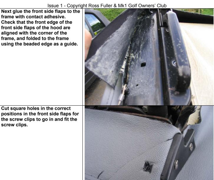
Cut square holes in the correct positions in the front side flaps for the screw clips to go in and fit the screw clips.
