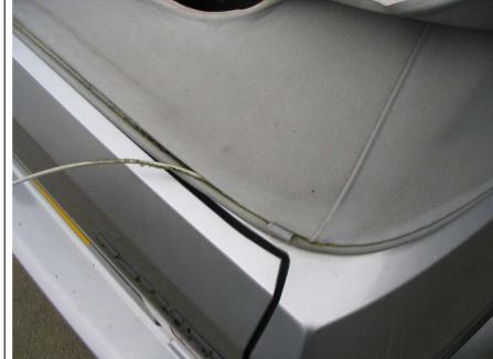
The hood should then be free from the car! Your half way there! Reattach the hydraulic strut so you can open the hood for cleaning the frame etc without doing any damage to the strut.
