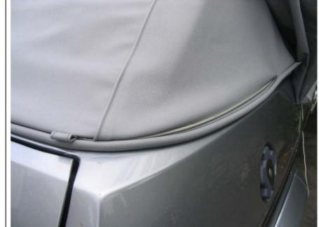
It will be a squeeze to get so much fabric under the lip in these places, so I shaped a bit of wood into a bolster chisel shape at one end to help it in, and used the flat end of the wood and a hammer to knock it in nicely.
