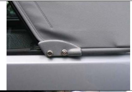
Feed the strap in the centre of the hood through the slits in the insulation layer. Double over the strap at the end to give it more strength and push the rivet through the strap then rivet it to the frame. Motorworld do a box of rivets and washers exactly the right size.
